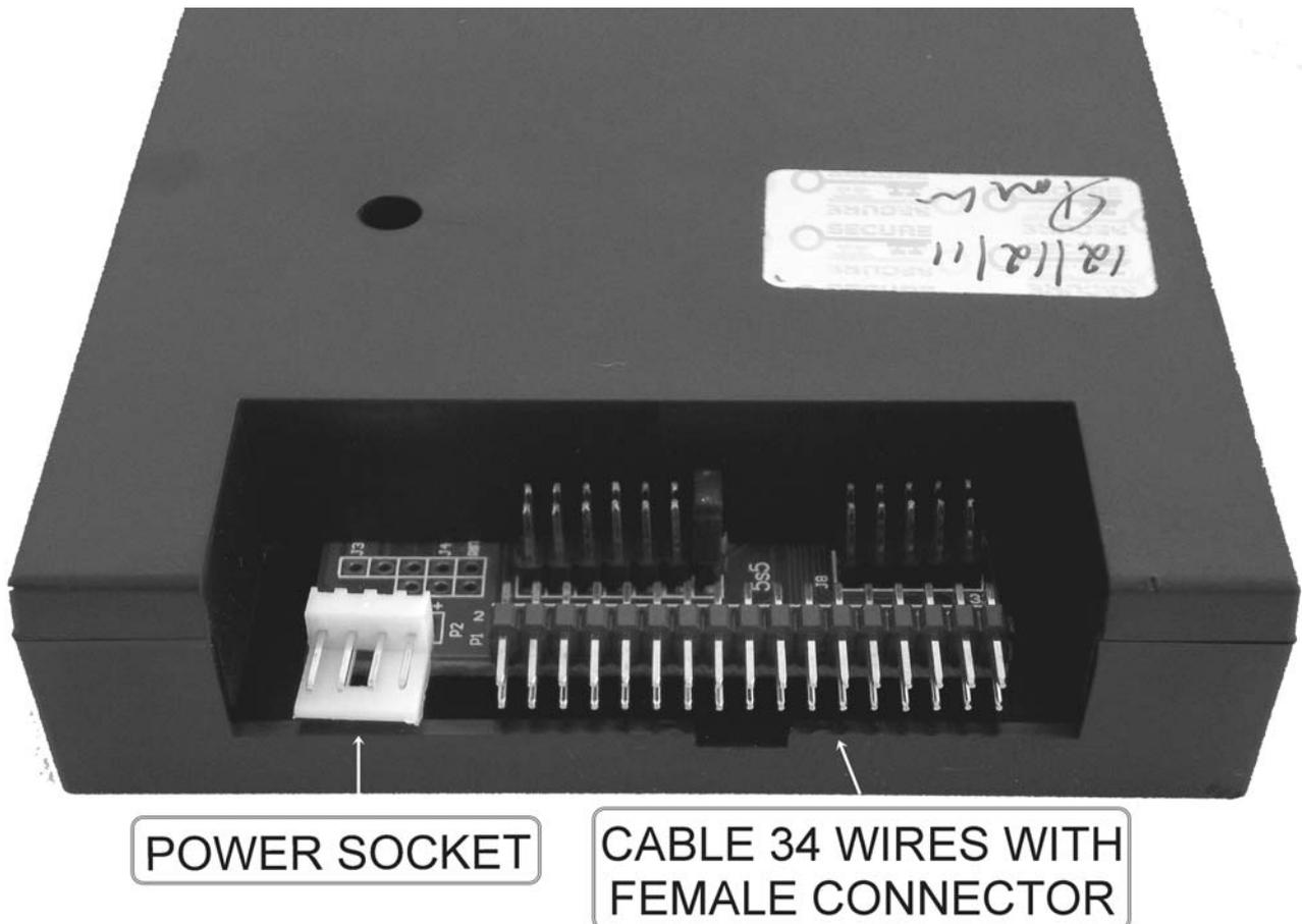
At the back of the USB disk drive you will find the connection for the voltage supply (+5V DC) and the 34 pin interface to connect the USB floppy disk drive controller. Please check for correct polarity of voltage supply when connecting the floppy USB disk drive.
